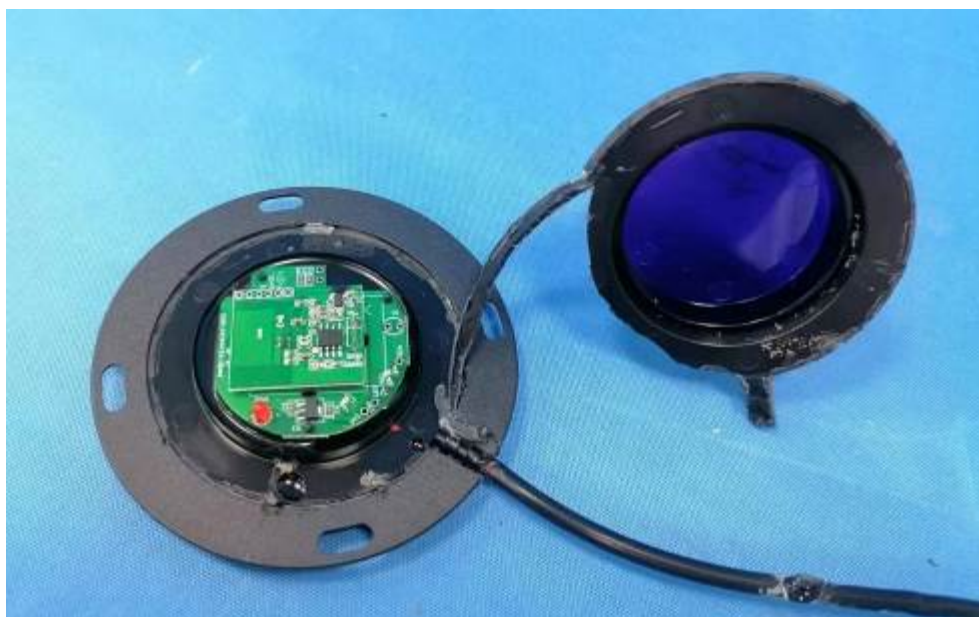
Internal view of sensor for FC-120
