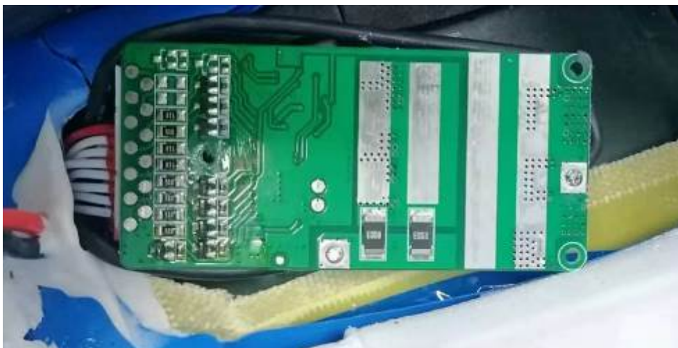
PCB of battery protection board view for W-100 and FC-120
