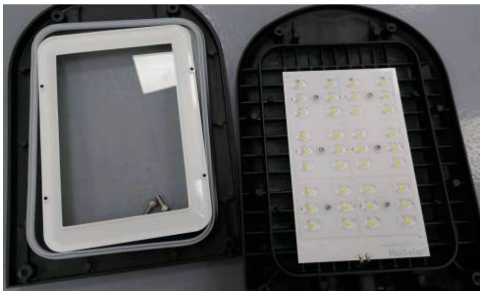
LED lens view of LED module for FC-120
