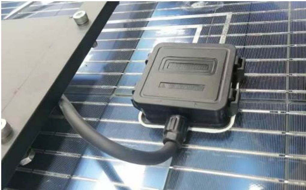
Lead wire of solar panel view for FC-120
