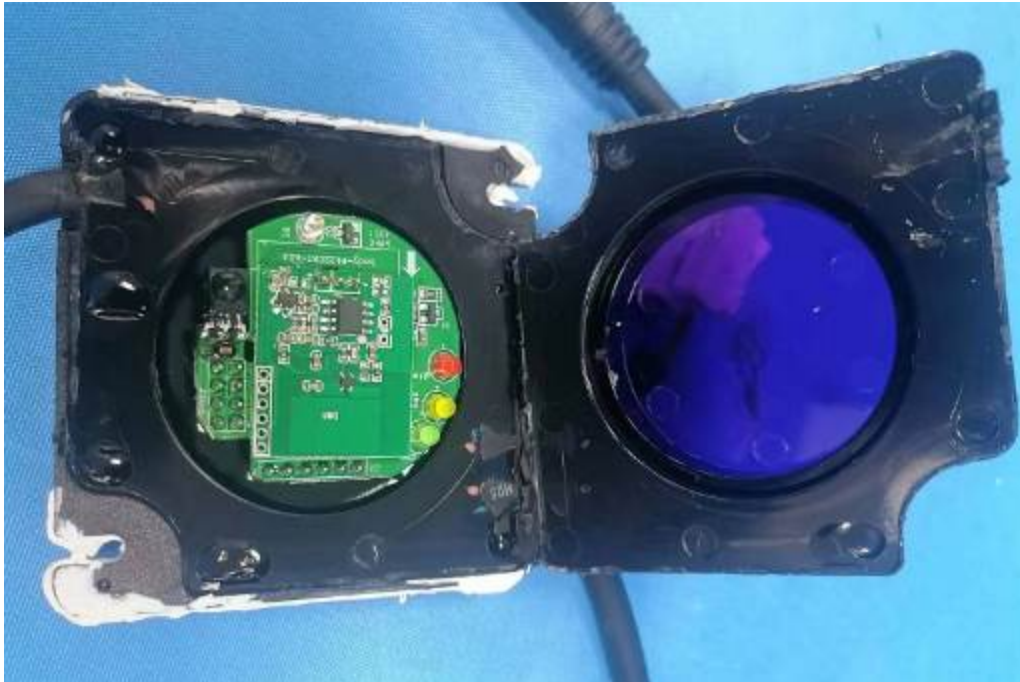
Internal of control device view for FC-60W
