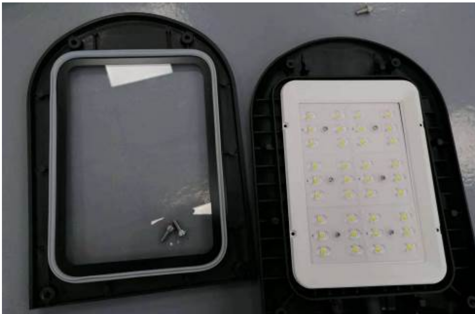
Internal view of LED module for FC-120
