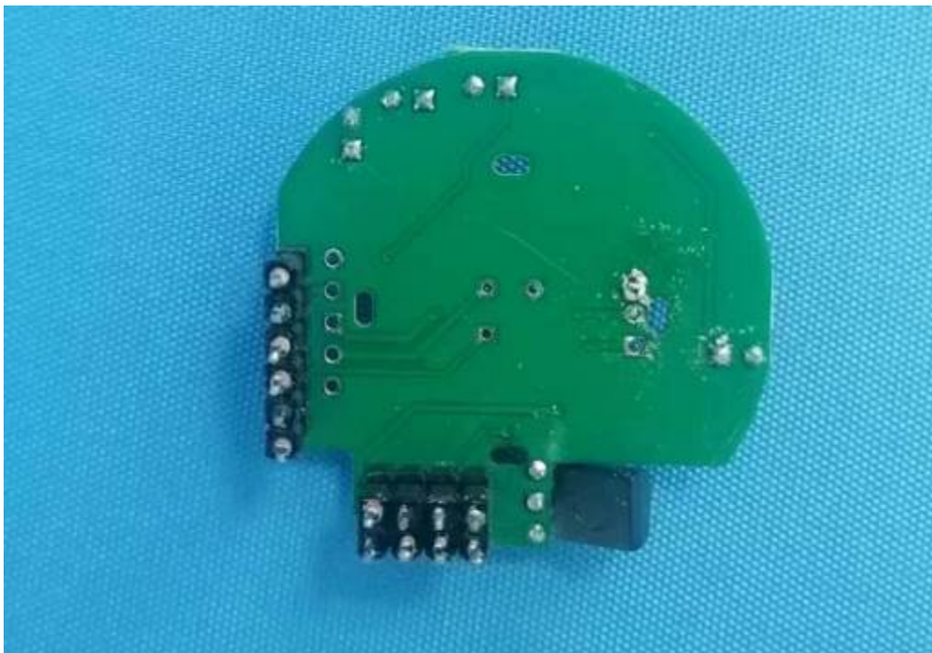
Son PCB view of control device for FC-60W
