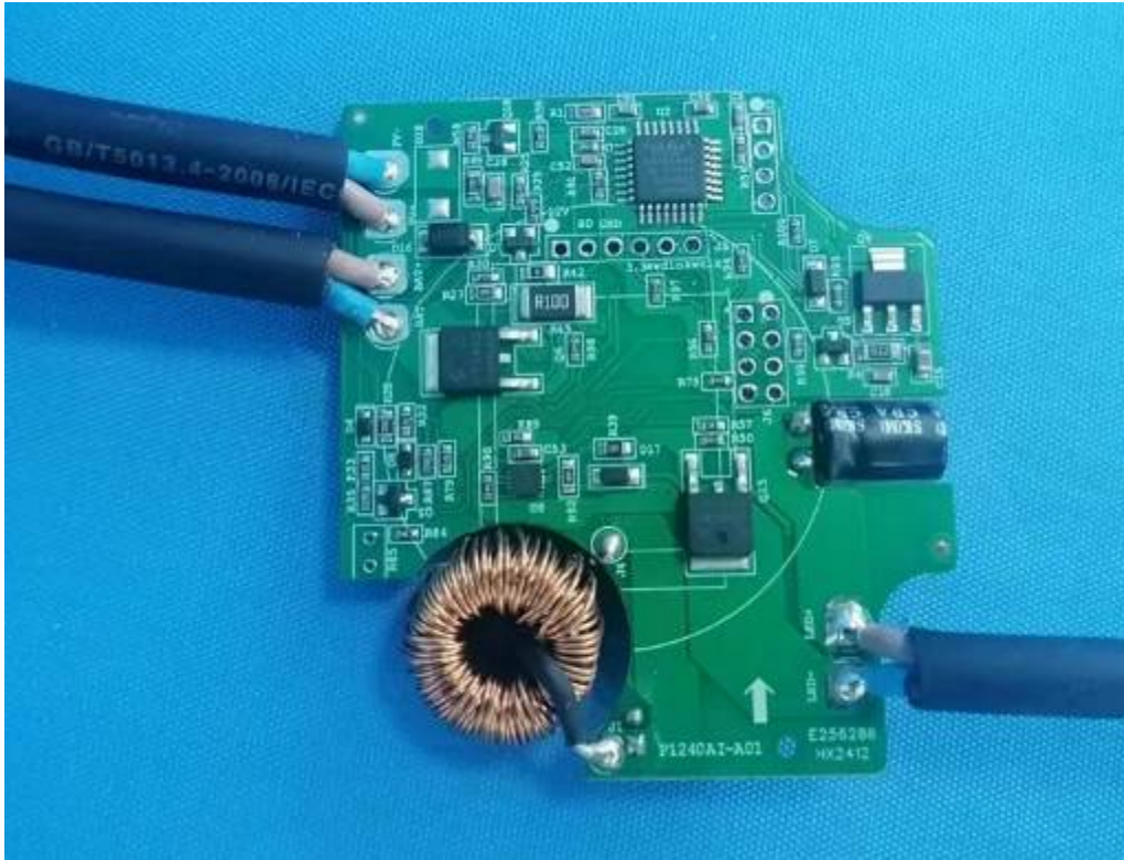
PCB view of control device for FC-60W
