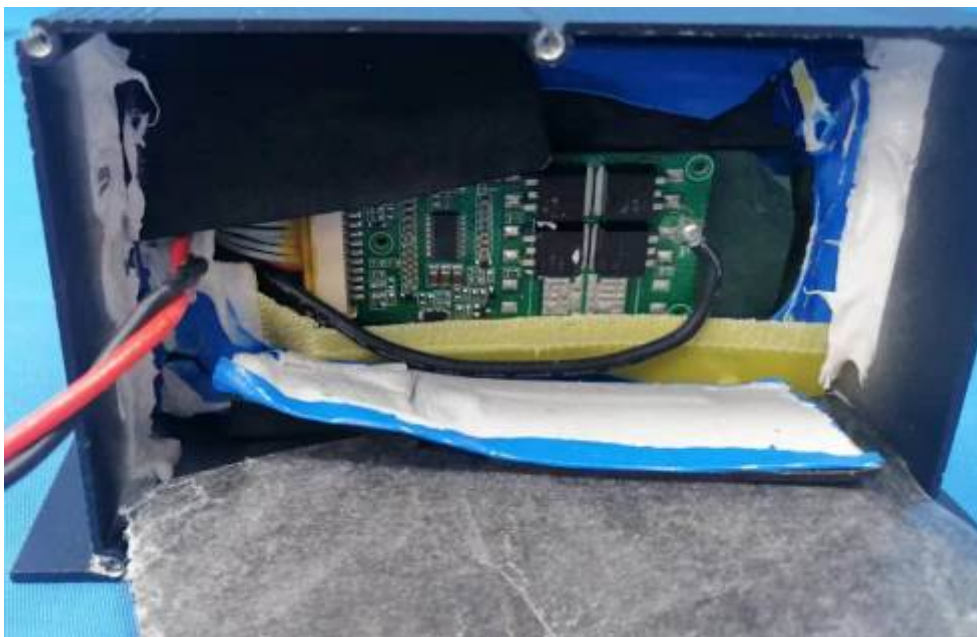
Battery protection board view for W-100 and FC-120
