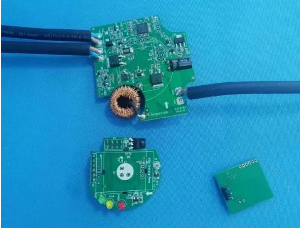
Explosive view of control device PCB for FC-60W
